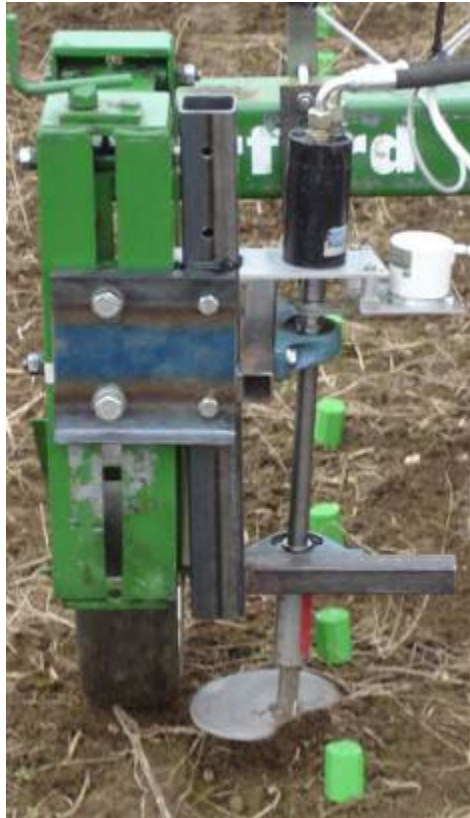
Figure 3 A single row field test rig with depth control and hydraulic drive shown operating on artificial plants above the soil surface.
