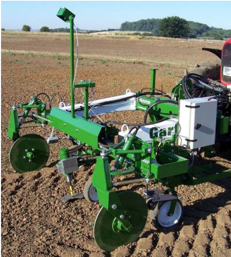
Figure 5 A 2m wide experimental toolframe designed and constructed by Garford Farm Machinery that will be used for all future trials and demonstration work.
