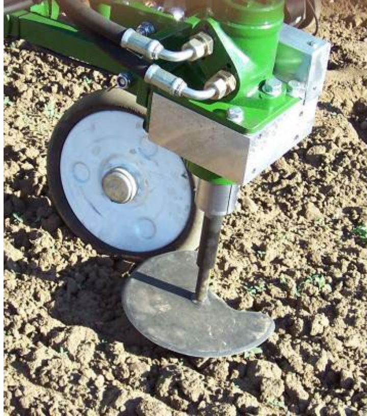
Figure 6 A hydraulically driven selective disc cultivation module fitted with a flat disc
