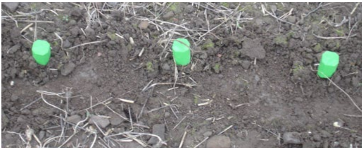
Figure 4 Cultivation between artificial plants at a 30 cm pitch using the rig illustrated in Figure 3
