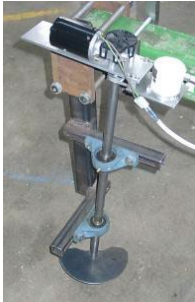
Figure 1: Electrically driven test rig for experimental development above ground
